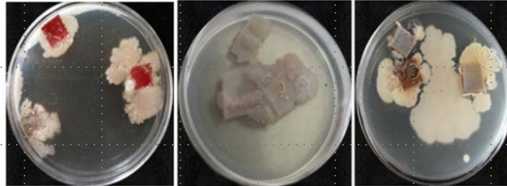
Fig. 1. Agar Flooding method. Growth of: a) bacteria on fries box B, b) parchment paper B, c) pizza box C.
